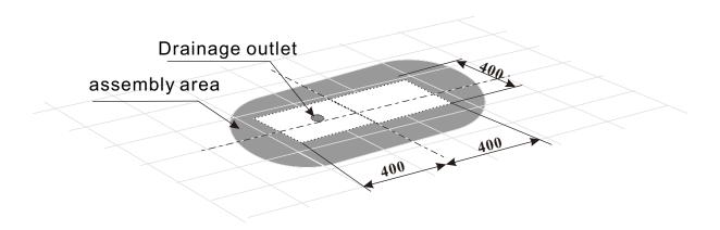
Remark: 1. Drainage outlet must be installed inside of the blank area.
